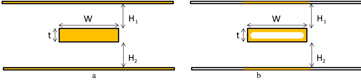
Figure 1. Conceptual sketch illustrating the current distribution (in yellow) within the cross section of a stripline with equidistant ground planes under DC conditions (a), and once the skin depth is smaller than the thickness of the trace (b).
