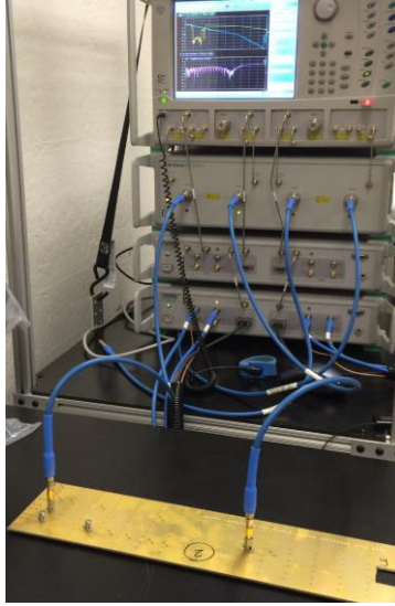
Figure 12. Setup configured to perform two-port S-parameter measurements.
