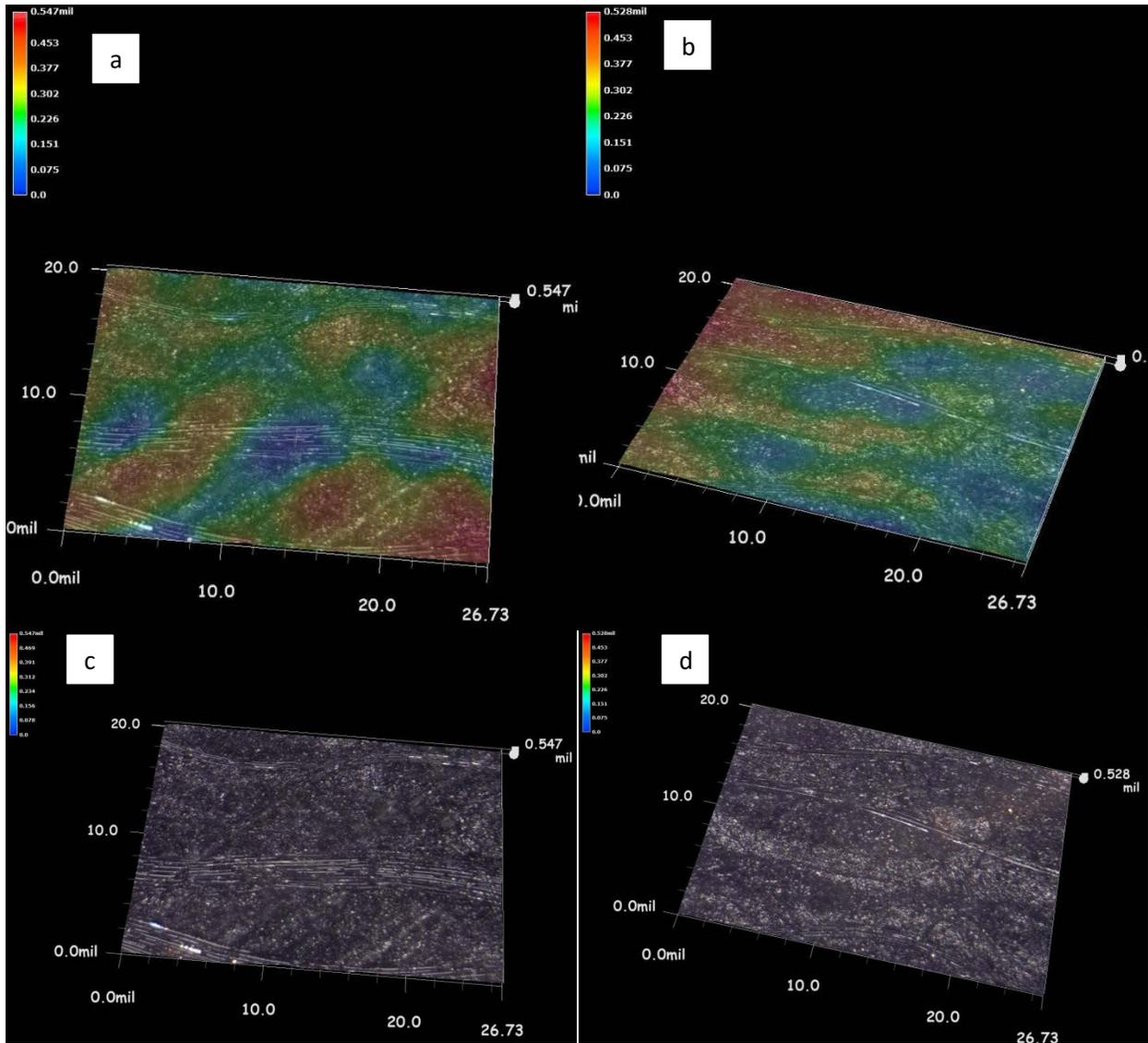
**Figure 6. Initial grinding (120 grit) of a sample mounted in epoxy using two different wheel speeds (150 and 300 rpm). (a) and (c) Sample ground at 300 rpm, (b) and (d) sample ground at 150 rpm. The images were taken using an optical microscope at 500X**
