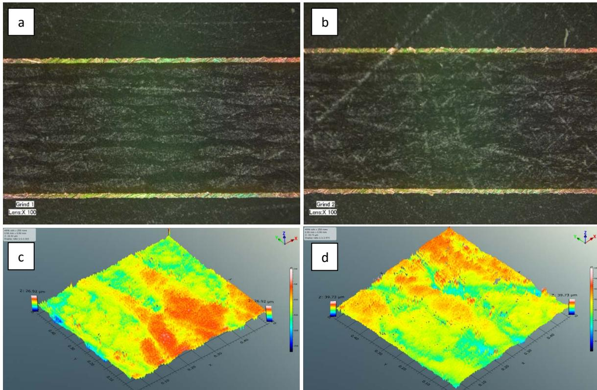
**Figure 4. Initial grinding (120 grit) of a sample mounted in epoxy using two different wheel speeds (150 and 300 rpm). (a) Sample ground at 150 rpm, (b) sample ground at 300 rpm, (c) detail of the topography of sample shown in (a), (d) detail of the topography of sample shown in (b)**
