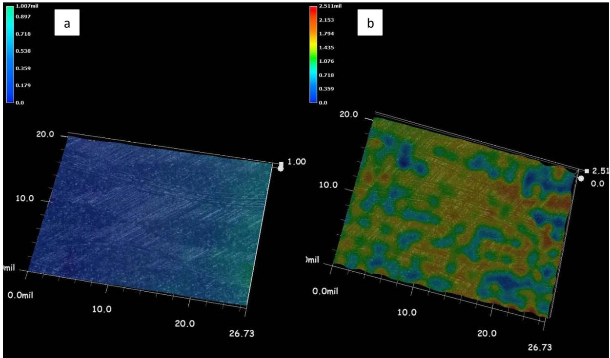
**Figure 7. Samples ground up to 1200 using two different wheel speeds (150 and 300 rpm). (a) Sample ground at 150 rpm, and (b) sample ground at 300 rpm. The images were taken using an optical microscope at 500X**
