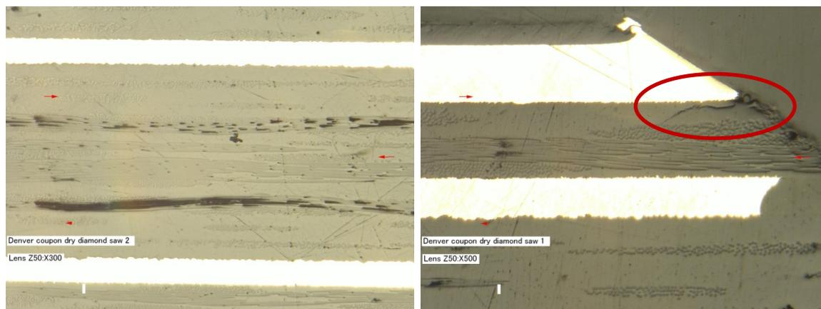
**Figure 1. Details of defects generated from inadequate sectioning: (a) excessive fiber pull-out and (b) crack at the edge of the sample. Samples were cut using a dry diamond saw and mount in acrylic. The samples were ground and polished using SiC papers: 180, 320, 500 and 1200 grit; 9 and 6 microns diamond and 1 micron alumina.**
