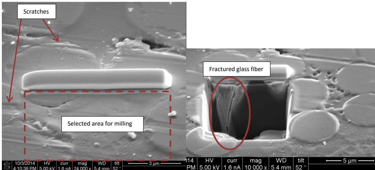
**Figure 9. Selected area of polished surface for focused ion beam (FIB). Damage on the fiber glass was observed after ion milling.**
