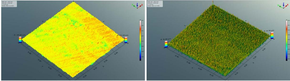
**Figure 8. Profilometer images for a sample ground/polished up to: (a) 500 grit (1 min) and (b) 1200 grit (20 s). Note that the surface seems fairly uniform and that the difference in height drops from 15.49 microns to 8.39 microns.**
