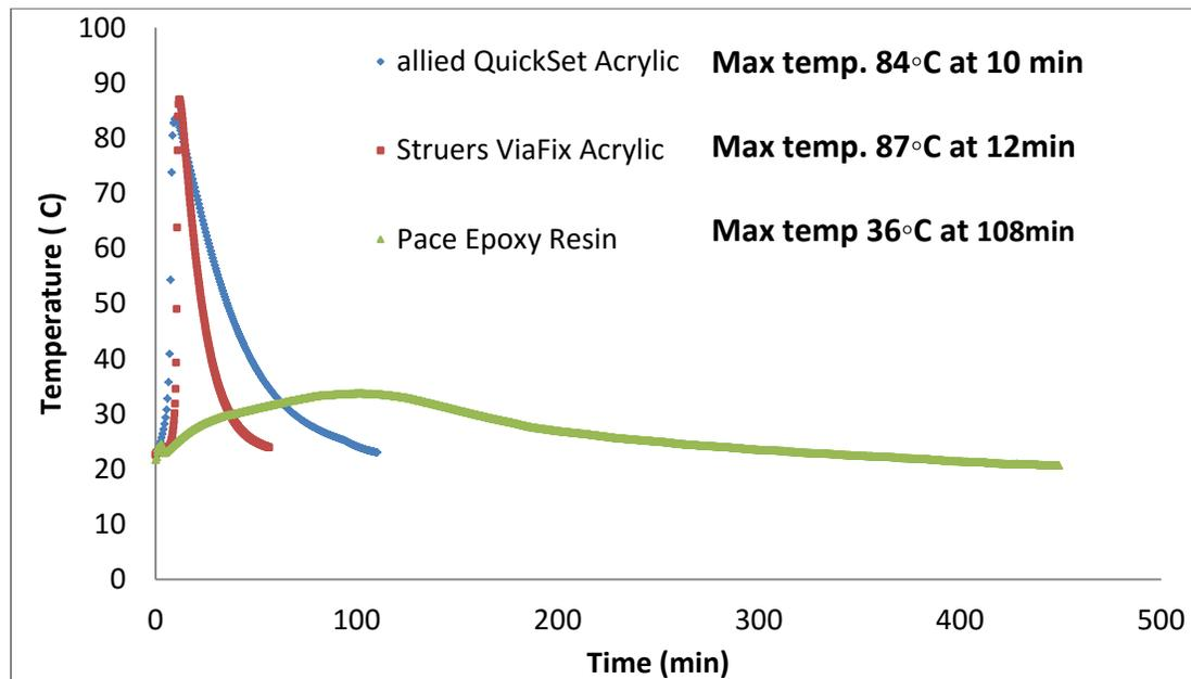
**Figure 3. Temperature versus time curves for laminates mounted in acrylic and epoxy.**
