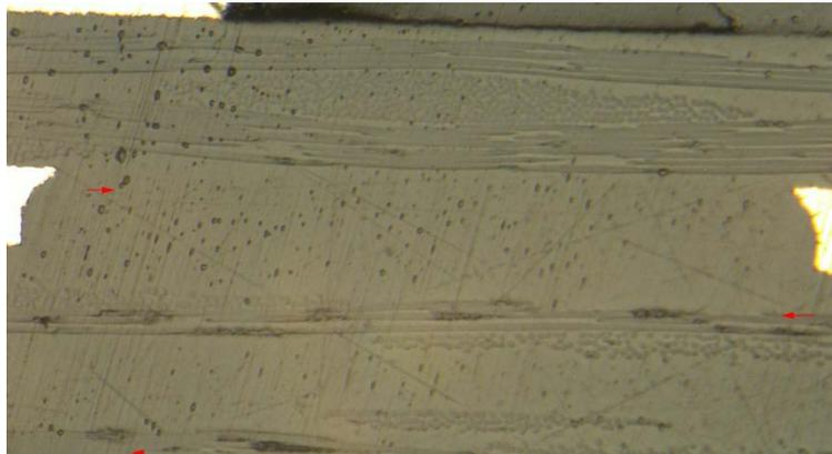
**Figure 2. Details of surface finishing after sectioning coupon using router. The sample was prepared using the same procedure as figure 1b.**
