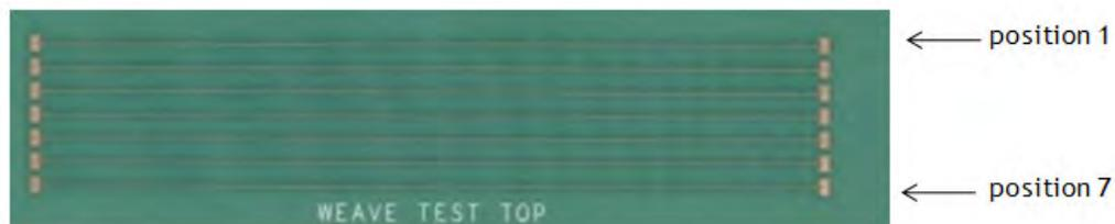
**Figure 22:** Microstrips located at different positions within the board.
