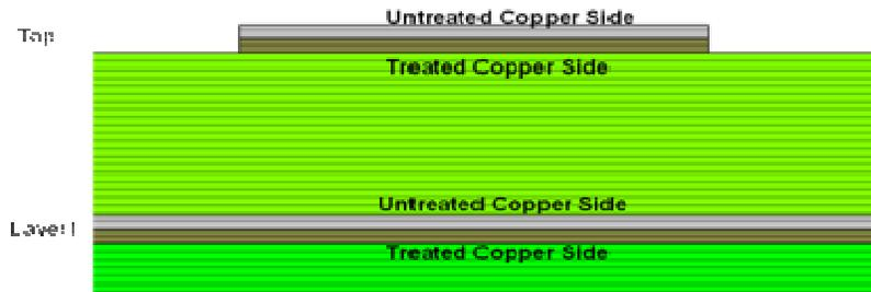
Figure 28: Copper “stack-up”.
