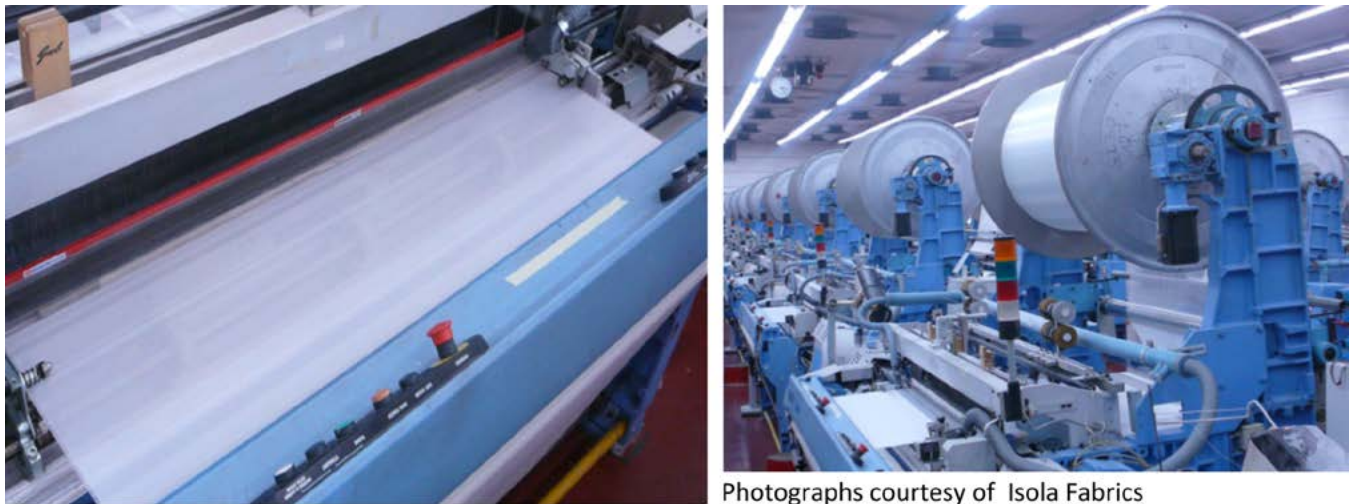
Figure 3: Glass weaving process.
