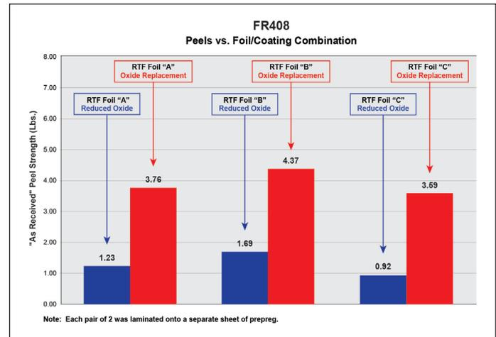
If reduced oxides are used, consult the chemical supplier for post oxide baking considerations as excessive baking may lead to lower pink ring resistance. It is generally suggested that post-oxide baking be performed vertically, in racks. Suggest mild bake of oxidized innerlayers (15-30 minutes @ 80-100°C).
