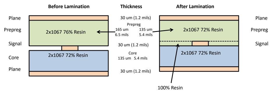
In this approach, the initial prepreg resin content is high, above the target, but after the resin loss into the circuit area, the structure is nearly balanced. Note-This is an example, the 76% prepreg may not be feasible to make. This also helps to show how high resin content structures can be hard to make balanced.
