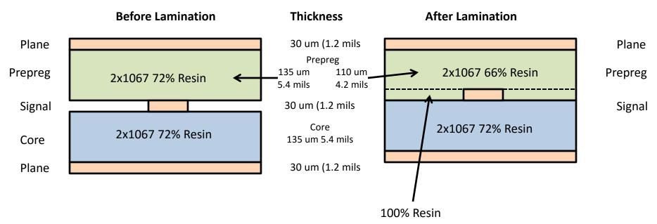
During lamination, the prepreg melts and flows into the areas around copper etched feature. In most SITVs the copper area is very small, so the resin requirement to fill this space is about 90-95% of copper thickness. This outflow of resin lowers the resin content of the prepreg layer, above the copper layer. The "effective resin content" in this case, is 66%, not 72%. In example above the resin content is reduced about 6%
