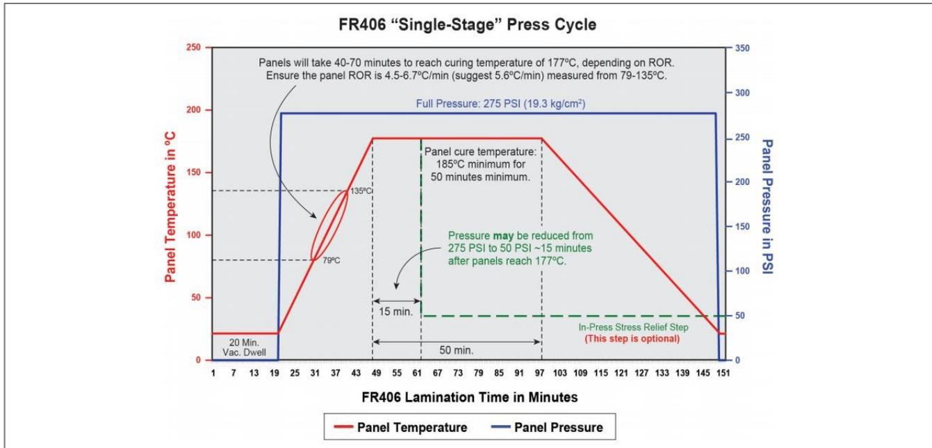
**Please note: This is not a press control program!** The graph represents the preferred pressure/temperature profile panels are subjected to during the lamination program cycle. **Note that the actual high pressure setting and cure duration chosen may differ from the 275 PSI suggested setting shown in this graph. Press pressure and cure duration selected may depend upon board design as well as other factors.**
