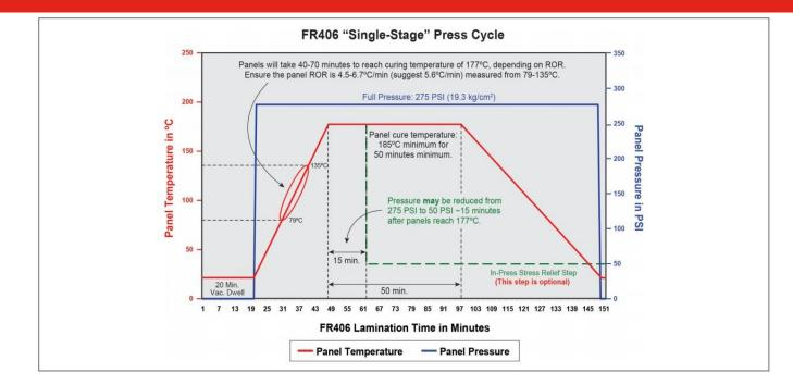
Please note: This is not a press control program! The graph represents the preferred pressure/temperature profile panels are subjected to during the lamination program cycle. Note that the actual high pressure setting and cure duration chosen may differ from the 275 PSI suggested setting shown in this graph. Press pressure and cure duration selected may depend upon board design as well as other factors.
