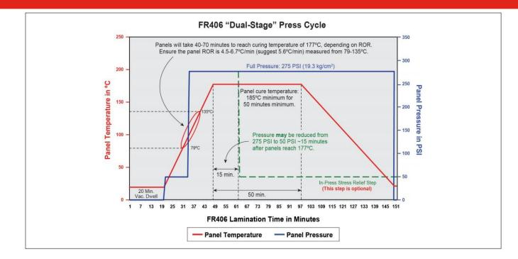
Please note: This is not a press control program! The graph represents the preferred pressure/temperature profile panels are subjected to during the lamination program cycle. Note that the actual high pressure setting and cure duration chosen may differ
